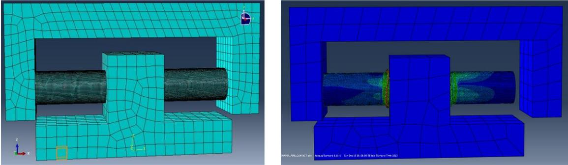
Fig. 6. Horizontal steel pipes as secondary dampers (axial crushing)
