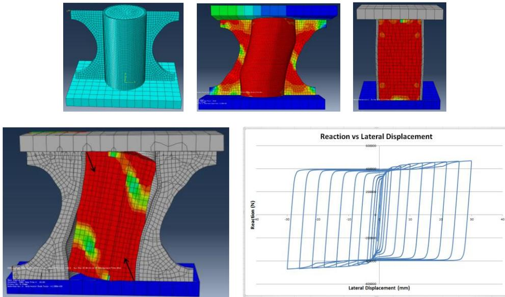
Fig. 3. Vertical steel pipe dampers: strengthened with tapered plates and lead filled inside the pipe (upper support plate is not shown). It can be seen that the lead reduce the buckle at the middle part of the pipe and dissipate energy through diagonal compression strut.
