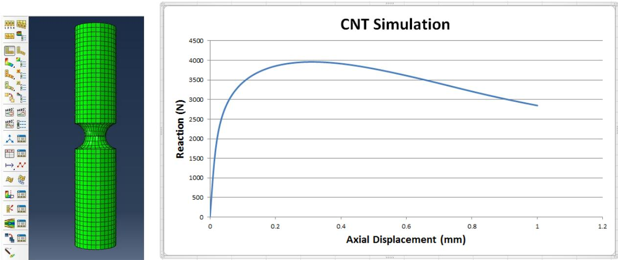
Fig. 7. Circumferentially notched tension bar (CNT) simulation
