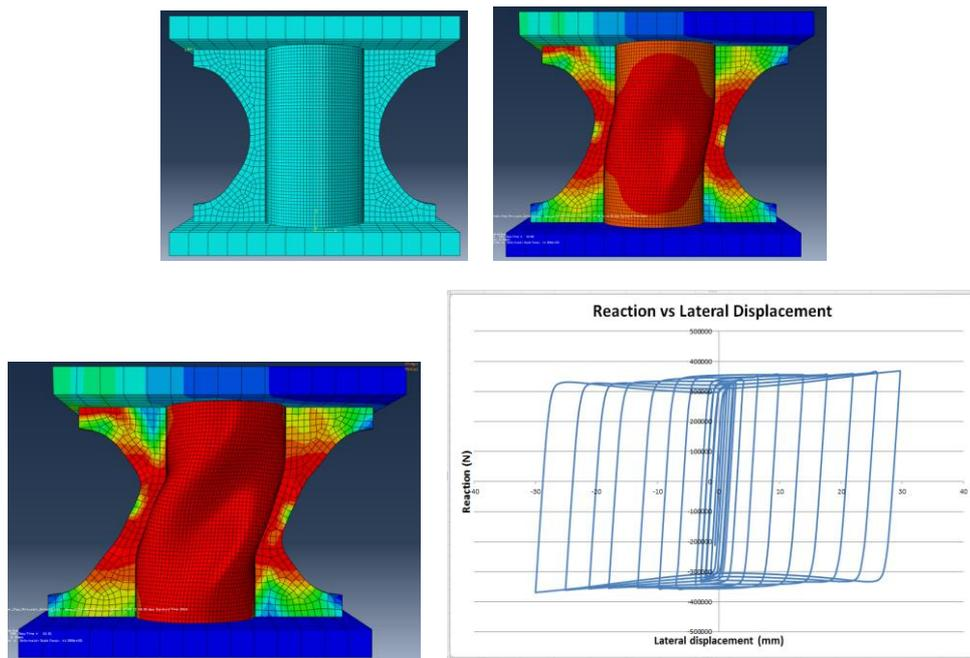
Fig. 2. Vertical steel pipe dampers: strengthened with tapered plates welded at outer sides of the pipe. The Mises plots are for 14 mm and 30 mm of lateral displacement. The tapered plates increase the capacity of the damper, however the middle part of the pipe buckles. The hysteresis behavior is better but the loop is still unstable.
