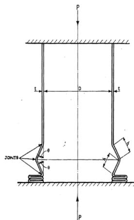
Fig. 5. Assumed collapse mode [3]
