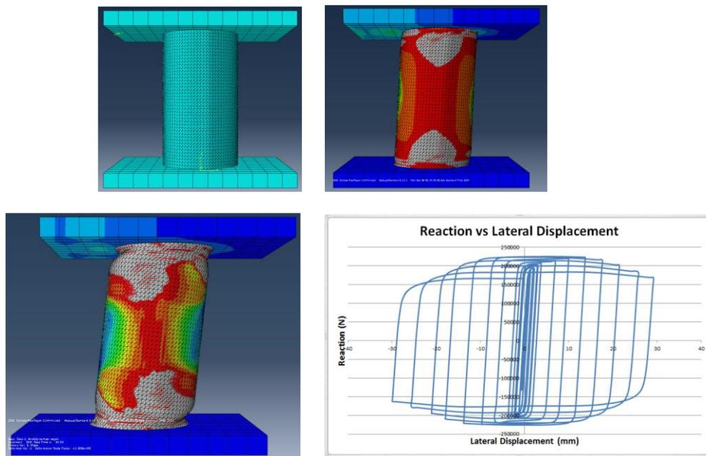
Fig. 1. Vertical steel pipe dampers: bare pipe damper. The Mises plots are for 14 mm and 30 mm of lateral displacement. Severe buckles occur at the top and bottom of the pipe at 30 mm lateral displacement. The hysteresis loop is fat but unstable.
