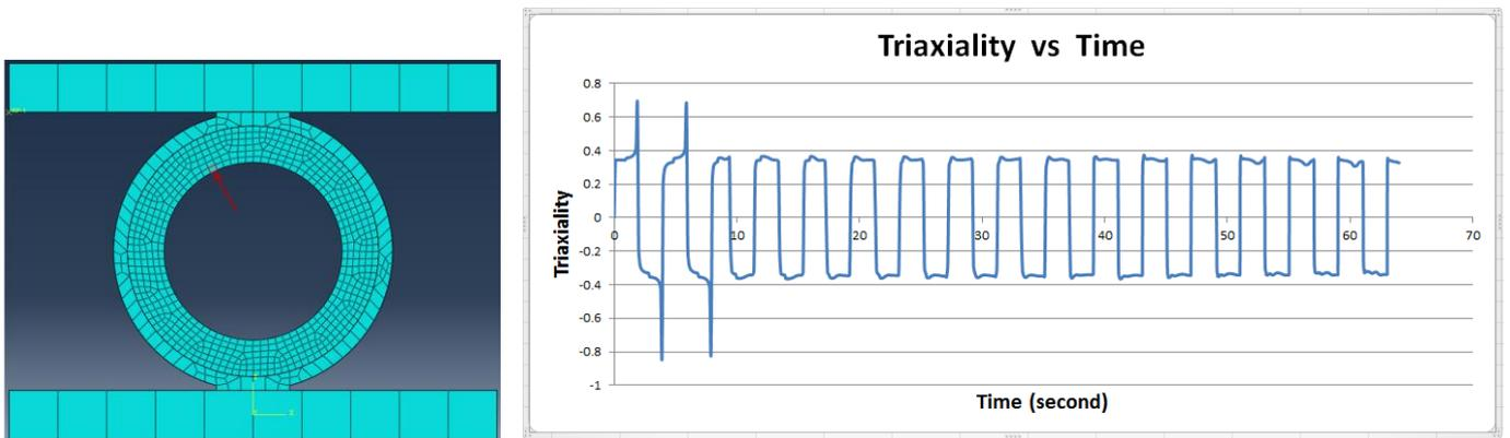
Fig. 8. Stress triaxiality vs time plot for the point of intense stress at the inner side of the ring (at the proximity of top and bottom supports). It can be seen in the right part of Fig. 8 that the stress triaxiality is constant ( $T \sim 0.35$ ). The micro voids due to cyclic deformation grow and shrink repeatedly in the ring-pipe damper.
