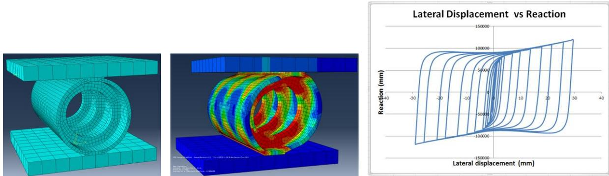
Fig. 4. Horizontal steel pipe dampers strengthened with three inner rings. The inner rings are welded to the pipe.
