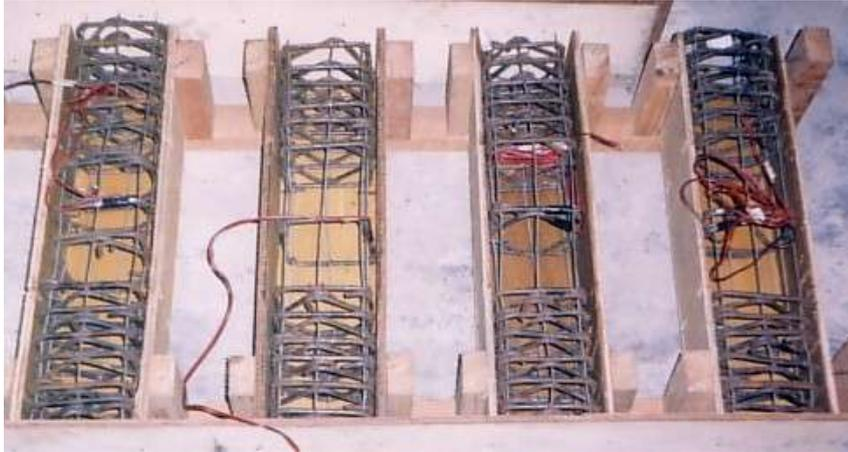
**Figure 3** Typical reinforcement cages for confined concrete.
