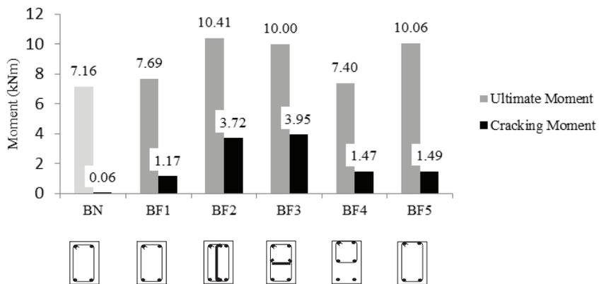
Fig. 2. Ultimate and cracking moment capacity
