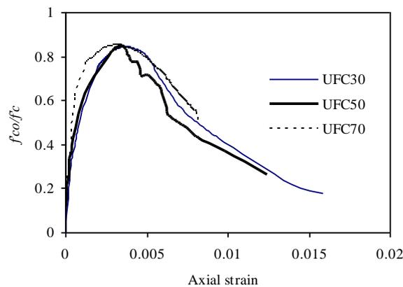
Figure 5 Stress-strain behavior of unconfined steel fiber-reinforced concrete
