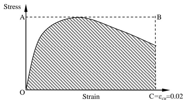
Figure 2 Toughness Index (Aoude et al., 2014)
