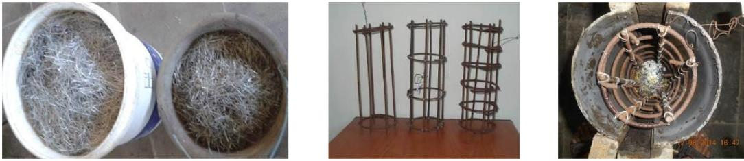
Figure 1 Steel fiber and reinforcement of specimens
