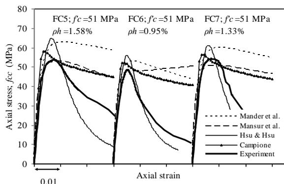
Figure 10. Comparison of confinement models with FC5, FC6, and FC7 specimens
