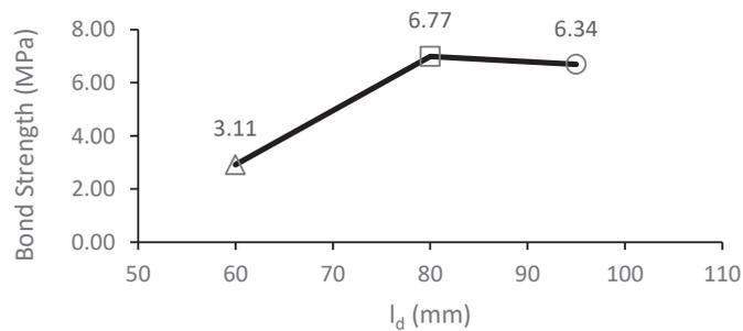
FIGURE 6. Bond strength with variation of bond lengths
