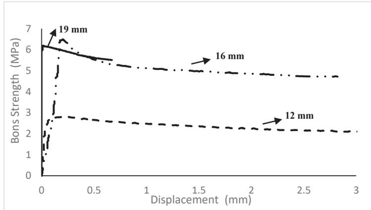
FIGURE 4. Bond Strength-Slip Curve
