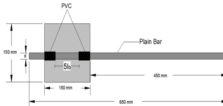
FIGURE 1. Pull Out Specimen
