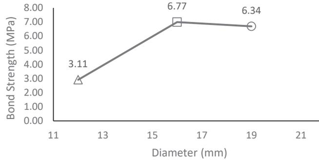
FIGURE 7. Bond Strength with variation of plain bar diameters
