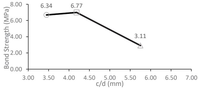
FIGURE 5. Bond Strength with variation of concrete cover to diameter ratio ( $c/d$ )
