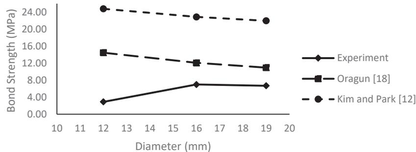
FIGURE 8. Comparison of bond strength generated from the equations.
