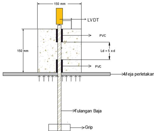
FIGURE 3. Setup of pull out test
