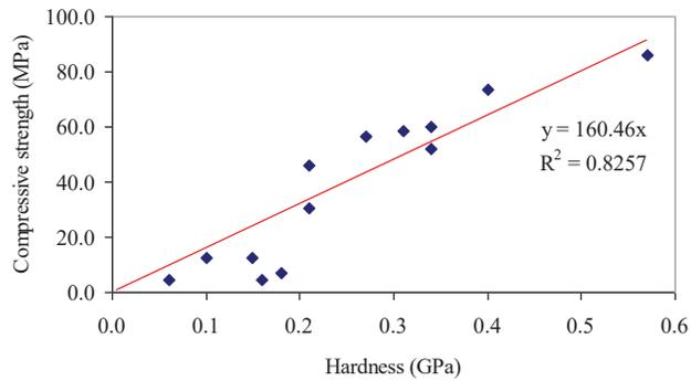
**FIGURE 9.** Vickers hardness versus compressive strength of geopolymers for all atomic ratios of Si:Al and Na:Al
