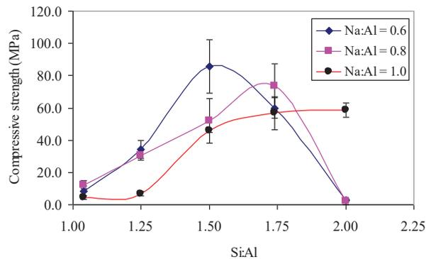
**FIGURE 7.** Compressive strength of geopolymers prepared with different initial ratios of Si:Al and Na:Al. Error bars represent 2SD.
