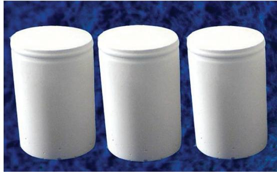
**FIGURE 1.** Metakaolin based geopolymers produced in this study.
