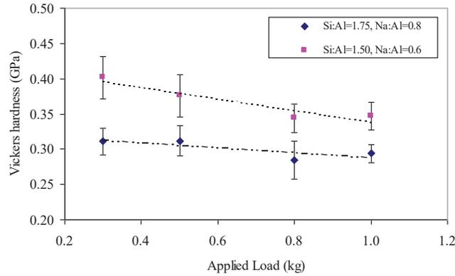
**FIGURE 2.** The dependence of hardness on the applied load with linear lines of best fit. Error bars represent 2SD.
