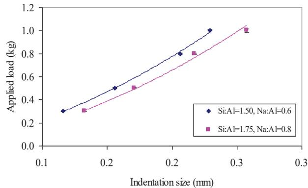
**FIGURE 3.** Indentation size ( $d$ ) as a function of applied load for geopolymer samples shown in Figure 2. The lines indicate the best-fit satisfying equation 4.
