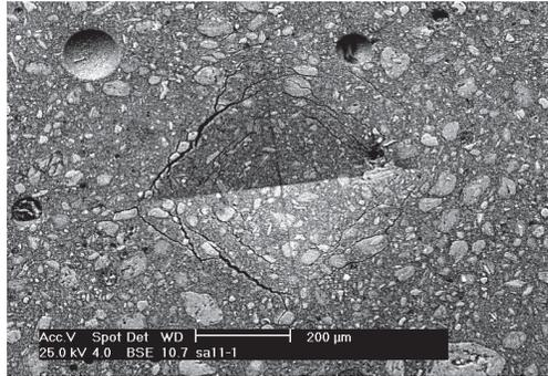
**FIGURE 4.** SEM micrograph of Vickers indentation of Si:Al = 1.04, Na:Al = 0.6 (load = 1 kg).
