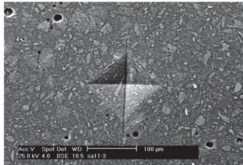
**FIGURE 5.** SEM micrograph of Vickers indentation of Si:Al = 1.5, Na:Al = 0.6 (load = 1 kg).
