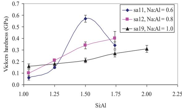
**FIGURE 6.** Vickers hardness as a function of Si:Al for three different values of Na:Al. Error bars repressed 2SD.
